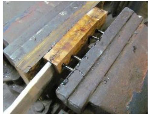
When done correctly, there will be pin stock visible on either side of the handle.
