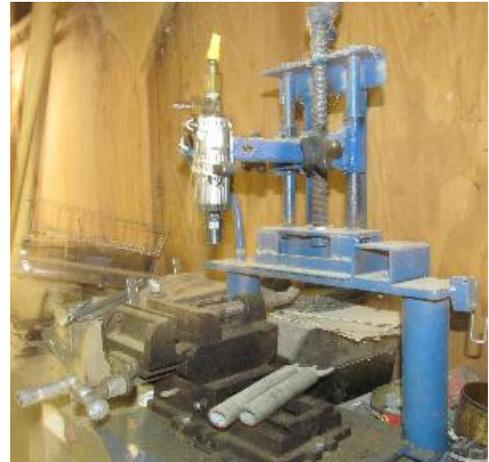
The shop vac and the mill are turned on and the recess is created. The best description of the process is "etch-a-sketch". Plow out the center well away from the lines, then come back and carefully run the edge of the end mill up to the line.
