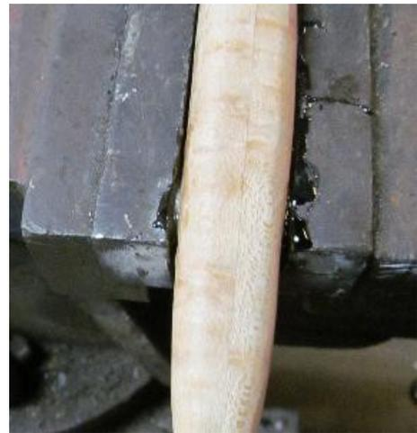
Use a rough grind to level the pins smooth to handle and then finish grinding the handle with 120, 320 and 600 grit belts.
