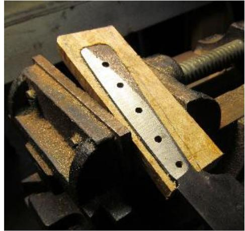
The tang is clamped into the recess and the pin holes are drilled. I use 1/8" pins. The holes in the tang are drilled with a #30 bit (0.128") so that there is allowance for slop in the pin diameter. As a precaution, I drill the scale holes with a #31 bit (0.120"). After epoxying the scales together, I will ream out the holes with a 0.125" bit. This process reduces the possibility of a pin hole being "wallowed" out and provides a tighter fit of pin to scale.
