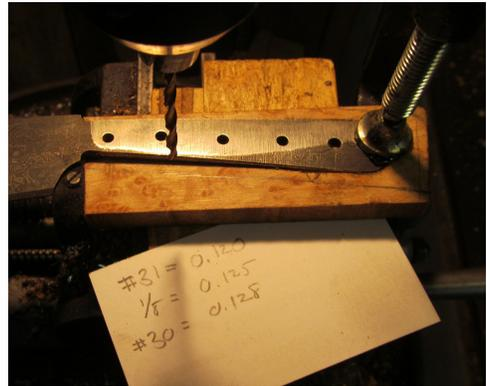
One of the realities of smithing (and knife making) is figuring out how to hold things. While C-clamps work, they are bulky. Old lab hose clamps actually work quite well. Alignment pins are very useful and are made from pin stock bent into 'L's and slightly ground to fit the #31 holes.
