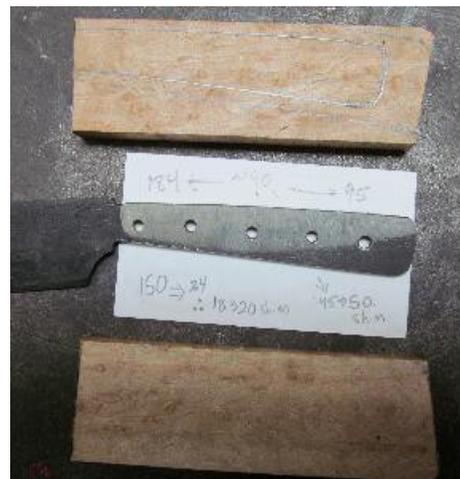
Shim stock can be used but so can old business cards (~0.010" thick). The appropriate number of thicknesses are positioned at the front spine and rear spine locations and the vise is closed. The end mill is positioned at the front spine location and the depth is set to 1/2 of the thickness of the tang at that location. Here that is 184, so 100 ought to do. Note that I round up a bit, usually 5 to 10 thousands. Afterall, the epoxy has to go somewhere.
