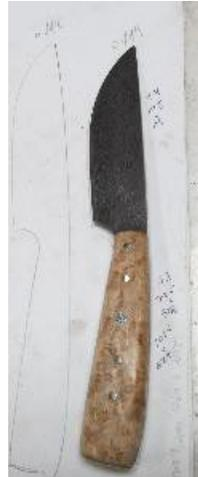
The last step is to coat the knife with hot beeswax. A heat gun is used to melt the wax and to heat the knife just hot enough to allow the wax to flow. Excess wax is wiped off and the handle is given a final buff with a cotton buff (no polish).
