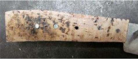
A coarse grind on the handle is accomplished with a rubber platen & an 80 grit AO flex belt.
