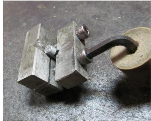
The pin stock is clamped in the pin vise with the mark visible. The vise is then placed on the vertical band saw and the pin is sawed as shown. This procedure is *sooo* much better than using a hack saw or a jewelers saw.
